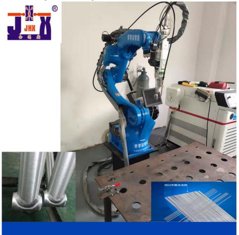
The welding products are aluminum, stainless steel and electronic metal components, which are thin or small and require higher welding requirements. Generally, laser welding robots can be used.
